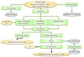
The traditional way of processing offals used to be wet-rendering (cooking under steam pressure) but it was replaced by dry-rendering, which resulted in meals of higher quality. The stabilized (or not) poultry offal is cooked/sterilized and dried down to 8% moisture. When the resulting meal appears to be too fat (above 16% fat), rancidity problems may occur during storage. Fat extraction is therefore recommended and yields a 10-12% fat content poultry by-product meal.
